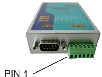
CNV300 Converter RS485 to TCP/IP Does not require installation. IP address set through Internet Browser(refer to CNV300 Manual)
