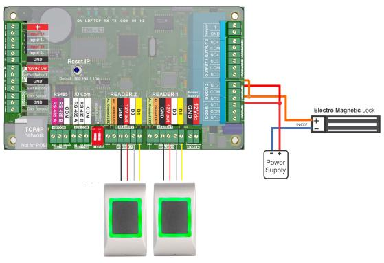
If Magnet is used connect the relays in parallel
