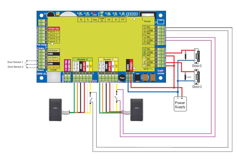
When card is presented on **Reader 1, Door 1** will open and in the same time **Free Output 2** will be activated for **60 seconds**. In this 60sec. Reader 2(Door 2) will be disabled. Furthermore, the readers will be in "Mantrap", which means that Door2 can not be open if Door 1 is still open. This all means that there are 2 conditions Door 2 to be open: Door 1 to be closed, and to pass X seconds from opening Door 1.
