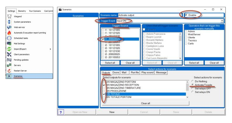
Select the trigger event to be "Input ON", then select which input and then select which outputs to be activated. In the end, select what will be the action on the output.
