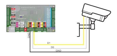
Connect the Wiegand output of the ANPR camera to the EWSi controller by connecting the wires D1, D0 and GND. The ground is necessary to be connected, since the camera is using different power supply.
