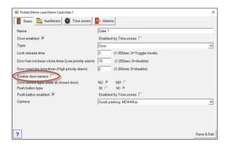
APB can work with or without door sensors. If it is with door sensors, then the APB is guided by the door sensor (if the door is physically open or not). If you don't use door sensors, then the APB is guided by the card punch itself.
