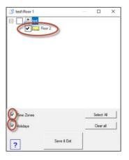
To transfer the same time zone to other controllers, right click on the controller and select "Copy settings to other controllers". Select to which controllers to be copied, then select both time zones and holidays if necessary. Go to Door/right click/Properties/Time zones tab.
